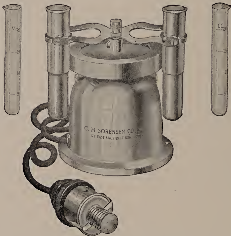
Fig. 3.—Small centrifuge adapted to chemical blood work.
